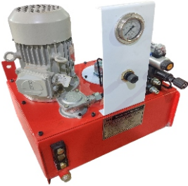
HYDRAULIC POWER PACK
